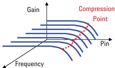
Figure 28. Compression measurements vs. frequency
