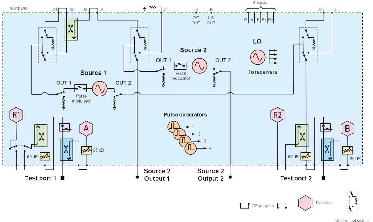
Figure 6. 13.5/26.5 GHz PNA-X block diagram with options 200, 219, 224, 020, 021, 022 and 025
