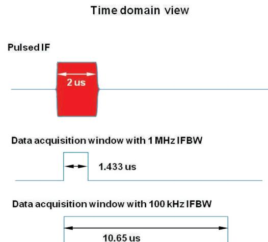
Figure 14a. Measurement errors caused by improper IF bandwidth
