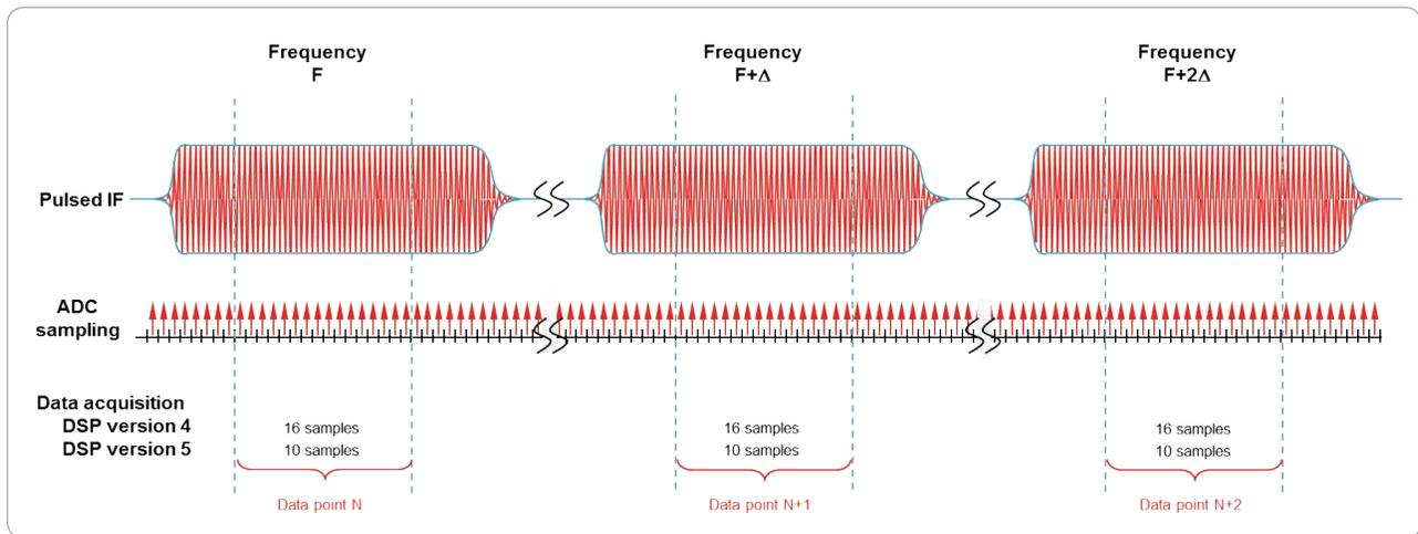
Figure 12. Wideband point-in-pulse and pulse-to-pulse data acquisition with widest IF bandwidth
