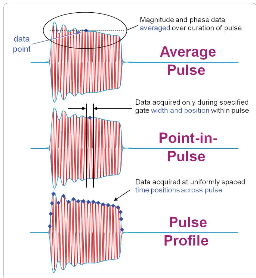
Figure 2. Average, point-in-pulse and pulse profile measurements
