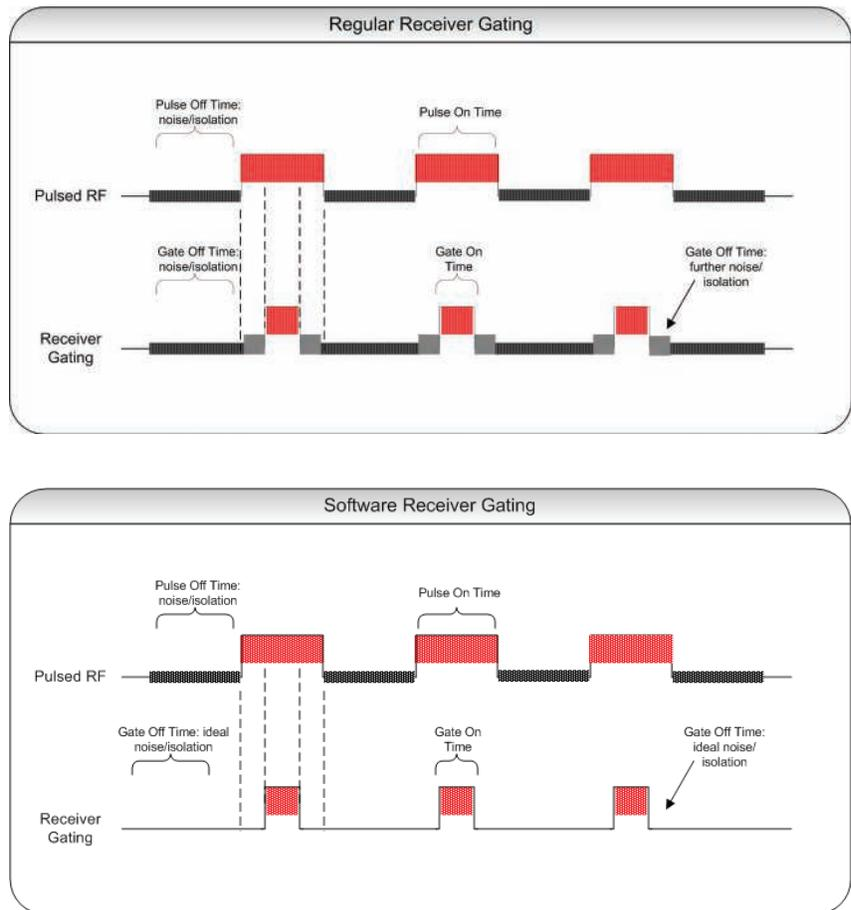
Figure 19. Software gating replaces the residual noise with ideal zeros and increases the receiver sensitivity
