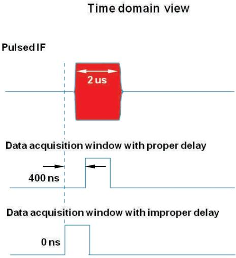
Figure 14b. Measurement errors caused by improper measurement delay
