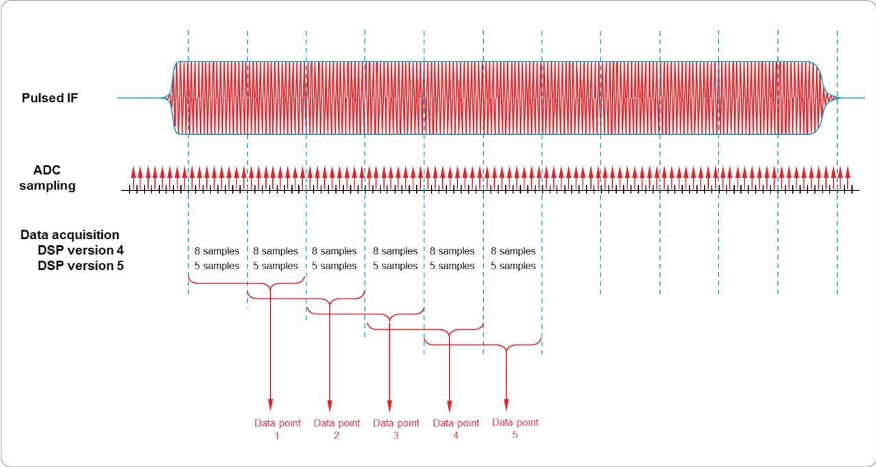
Figure 13. Wideband pulse profile data acquisition using widest IF bandwidth
