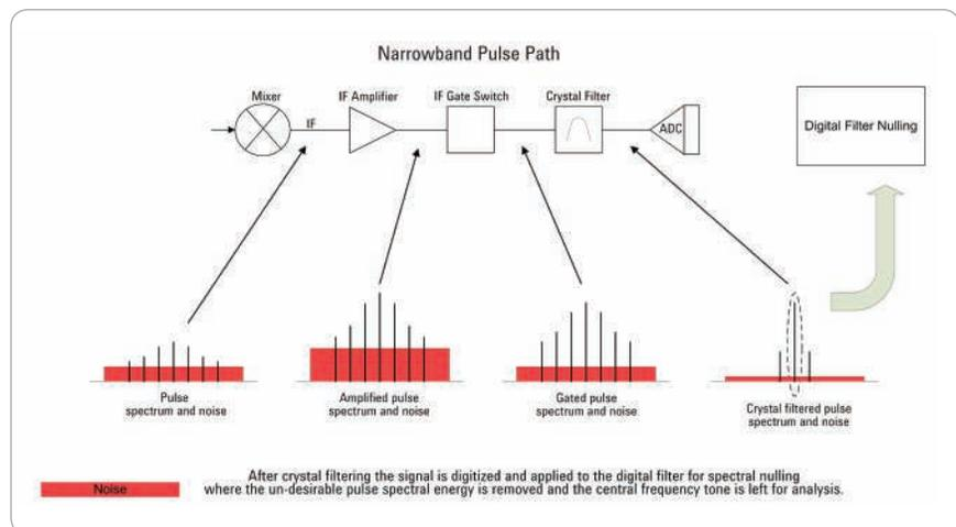
Figure 17. Narrowband filter path
