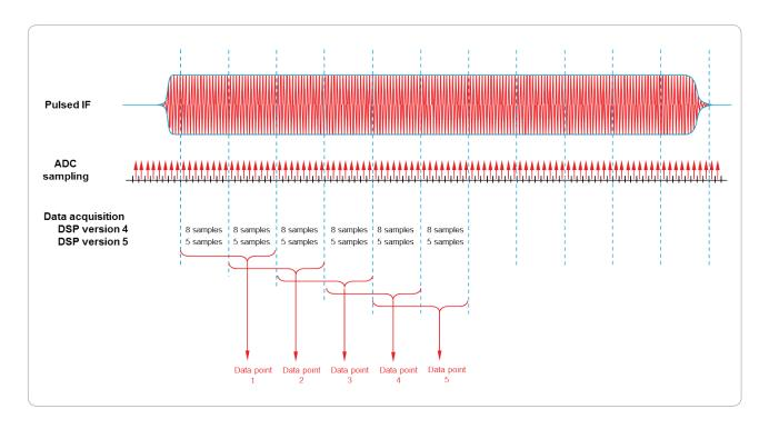
Figure 13. Wideband pulse profile data acquisition using widest IF bandwidth
