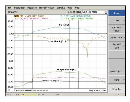
Figure 25a. Uncorrected narrowband pulse measurements
