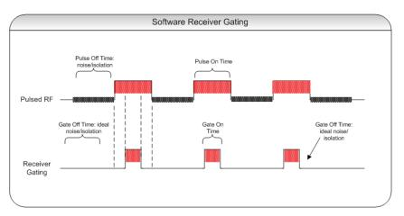
Figure 19. Software gating replaces the residual noise with ideal zeros and increases the receiver sensitivity
