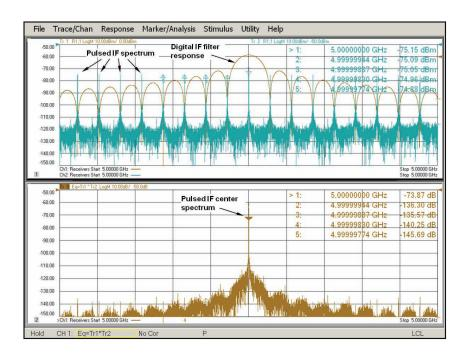
Figure 21. Filter nulling is used to reject undesired pulse spectrum
