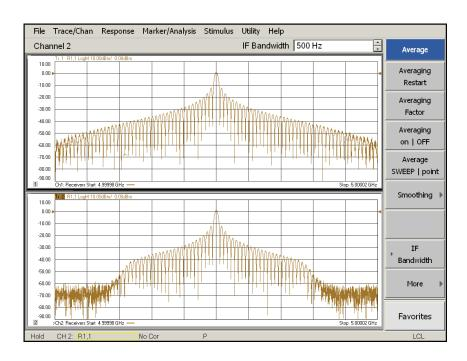
Figure 18. Pulsed-RF signal filtered in wideband IF path and narrowband filter
