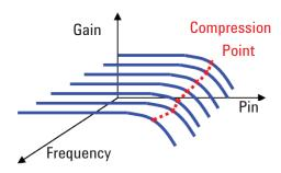
Figure 28. Compression measurements vs. frequency
