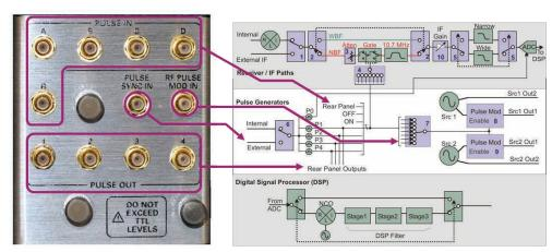
Figure 8. Rear panel pulse I/O
