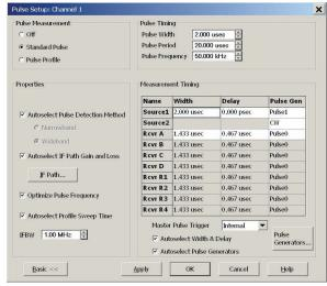
Figure 11b. Advanced Pulse Setup dialog box
