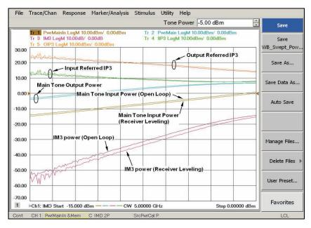
Figure 30c. Wideband pulse swept-power IMD measurement comparisons between open loop and receiver leveling
