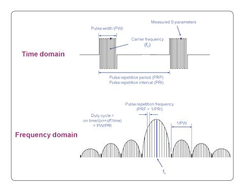
Figure 3. Pulsed-RF network analysis terminologies
