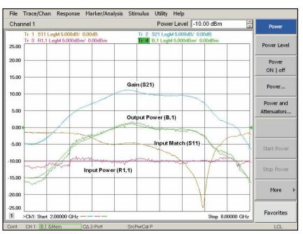
Figure 24. Calibrated wideband pulsed S-parameters and absolute power measurements with a comparison between open loop and receiver leveling modes
