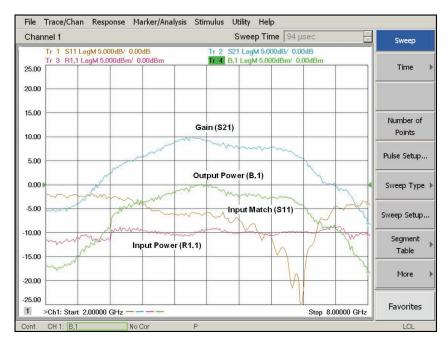
Figure 23. Uncorrected pulsed-RF S-parameters and absolute power measurements using wideband detection
