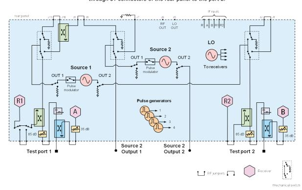
Figure 6. 13.5/26.5 GHz PNA-X block diagram with options 200, 219, 224, 020, 021, 022 and 025
