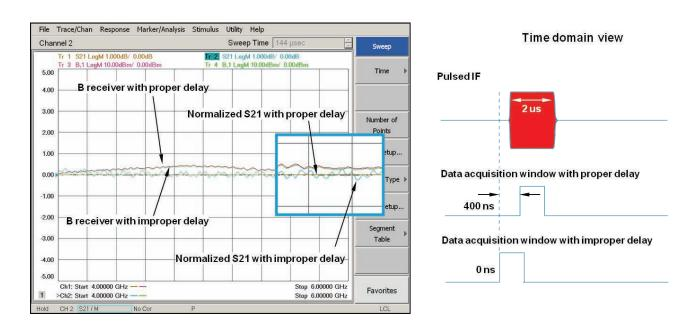
Figure 14b. Measurement errors caused by improper measurement delay
