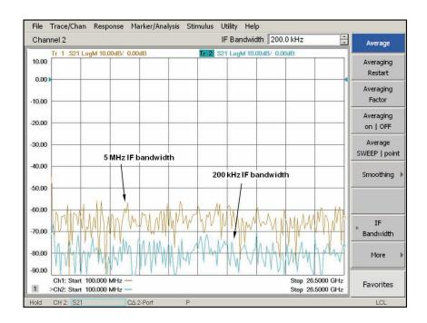
Figure 16. PNA-X wideband pulse measurement dynamic range
