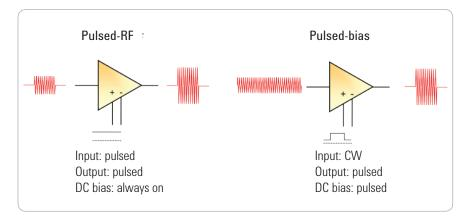
Figure 1. Pulsed-RF and pulsed-bias operation modes
