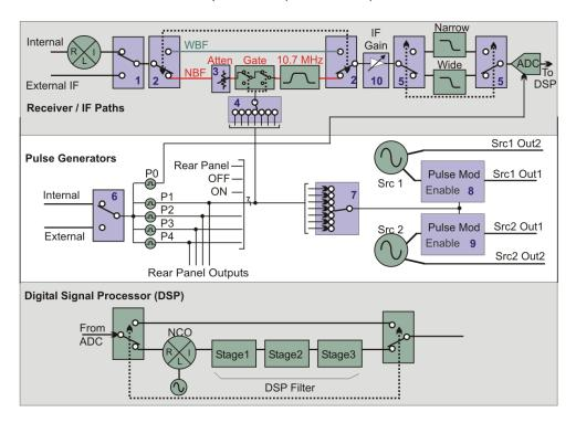
Figure 7. PNA-X IF path block diagram
