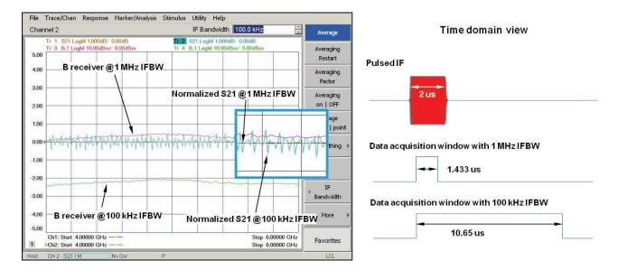
Figure 14a. Measurement errors caused by improper IF bandwidth
