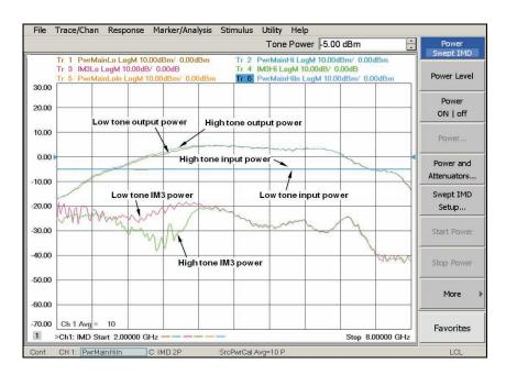
Figure 30b. Wideband pulse swept-frequency IMD measurements with receiver leveling
