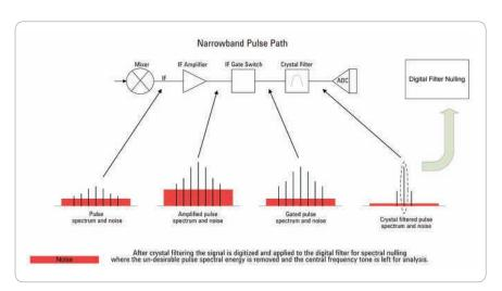
Figure 17. Narrowband filter path
