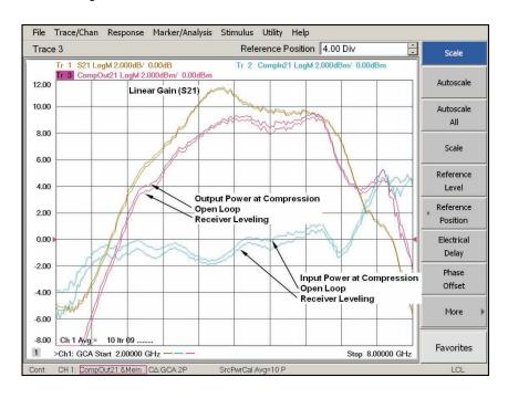
Figure 29. Wideband pulse GCA measurement comparisons between open loop and receiver leveling
