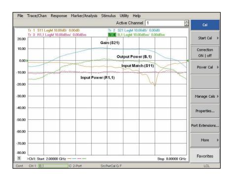
Figure 25b. Measurements after calibration with pulse modulator off
