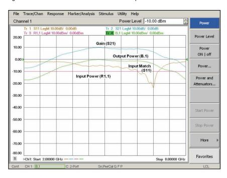
Figure 25c. Corrected pulsed-RF S-parameters and absolute power measurements using narrowband detection
