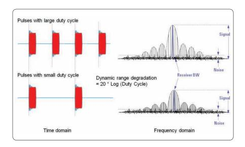
Figure 5. Duty cycle (time domain) versus signal-to-noise ratio of center spectrum (frequency domain)
